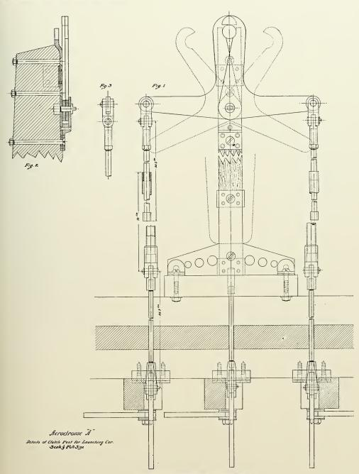
DETAILS OF CLUTCH POST FOR LAUNCHING-CAR
